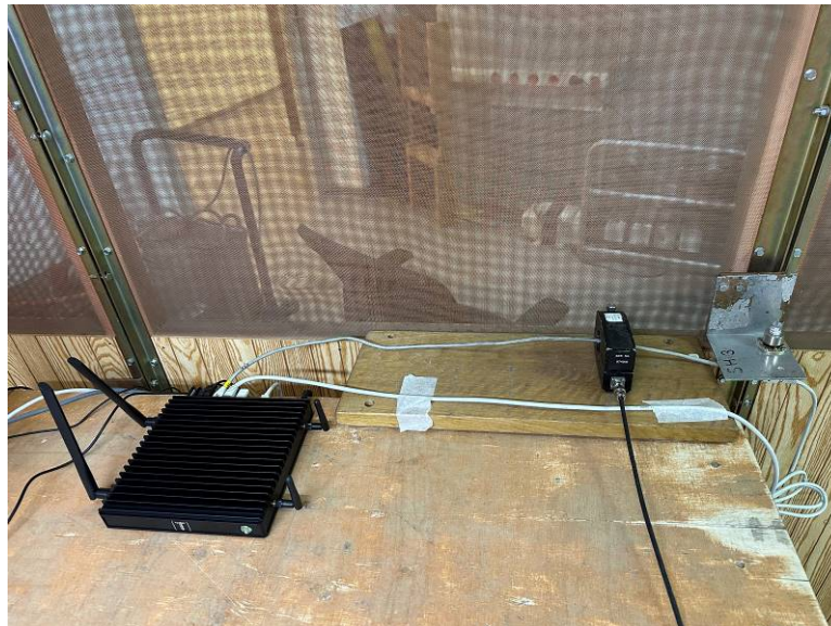
Photograph 8.2.1 Setup for conducted emission measurements at wired network port with current probe
