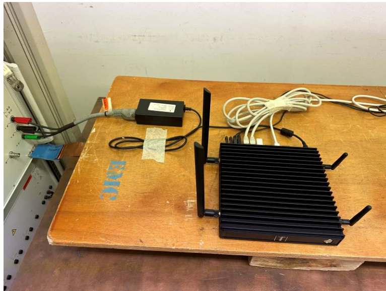
Photograph 10.7.1 Setup for immunity to voltage dips and short interruptions
