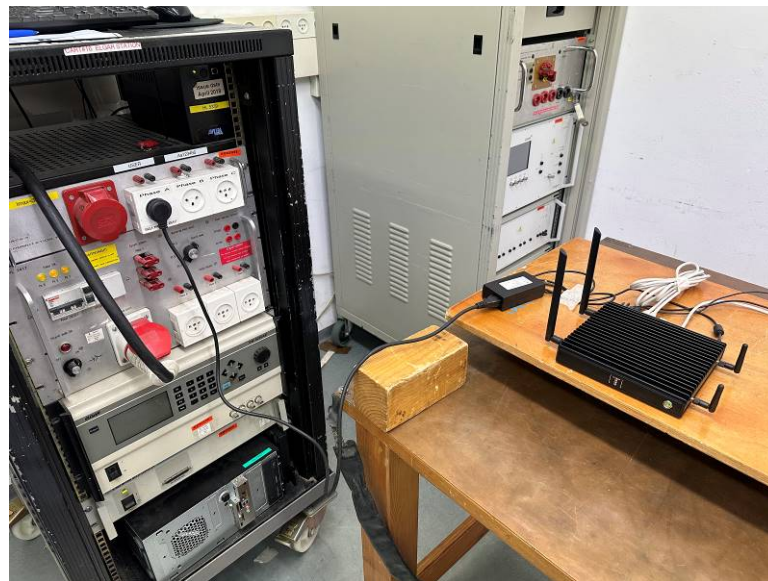
Photograph 9.5.1 Setup for voltage fluctuations and flicker test
