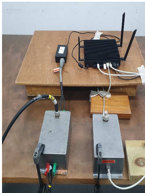
Photograph 10.5.1 Setup for immunity to conducted disturbances induced by RF fields at AC power supply line
